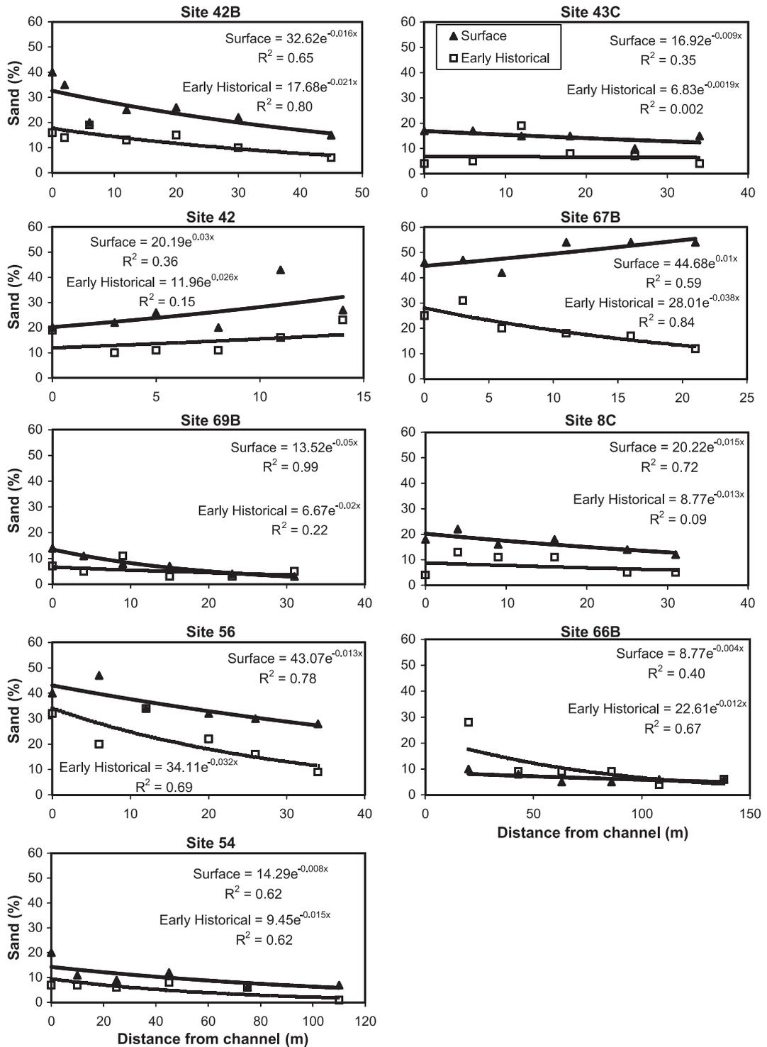
Fig. 6. Lateral changes in grain size at each cross-valley transect. Surface samples represent the upper 5–10 cm of each core. Early historical samples were collected from the first 2–10 cm of historical alluvium directly overlying the presettlement soil.
