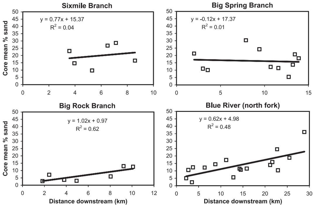
Fig. 4. Downstream changes in grain size for each reach. Data include depth-integrated composite samples of the entire thickness of the historical alluvium from bank exposures (data from Lecce, 1993).
