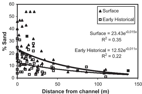
Fig. 5. Lateral changes in grain size for the entire watershed. Surface samples represent the upper 5–10 cm of each core. Early historical samples were collected from the first 2–10 cm of historical alluvium directly overlying the presettlement soil.
