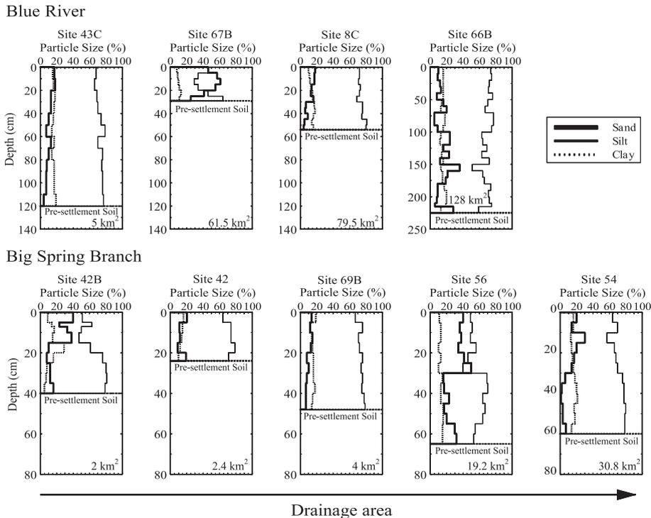
Fig. 2. Percentages of sand, silt, and clay in near-channel cores. Although these data only show vertical trends for near-channel cores, the coarsening-upward was also observed in almost every core across each flood plain transect.
